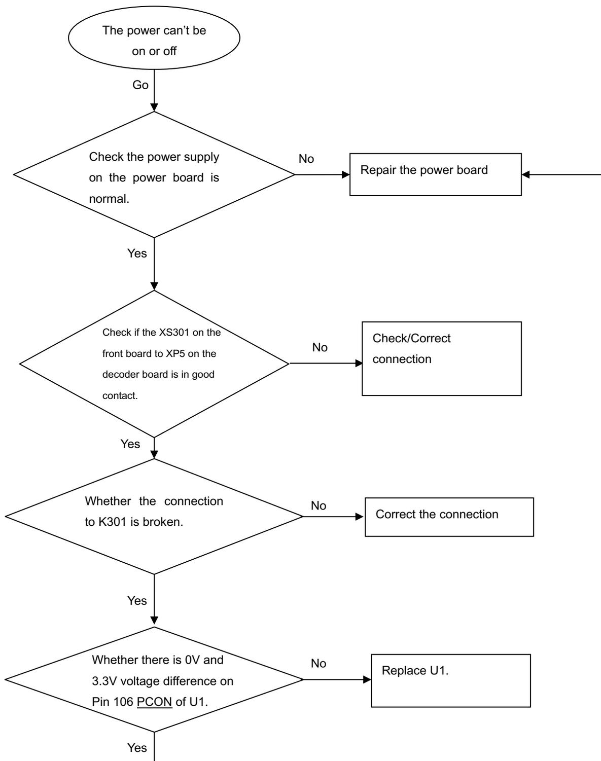
**All output voltages on the power board is 0V or deviated.**
